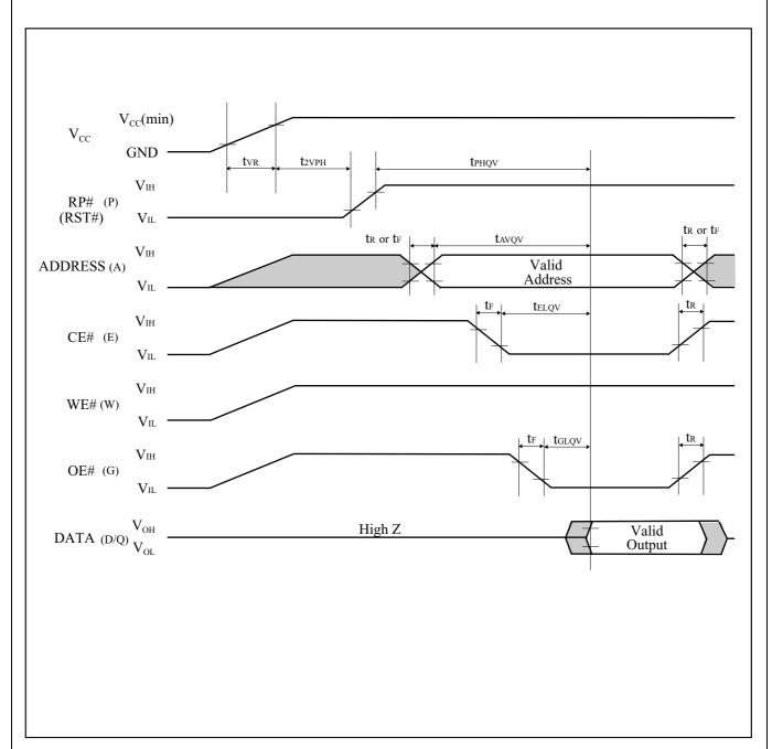
Figure A-1. AC Timing at Device Power-Up
