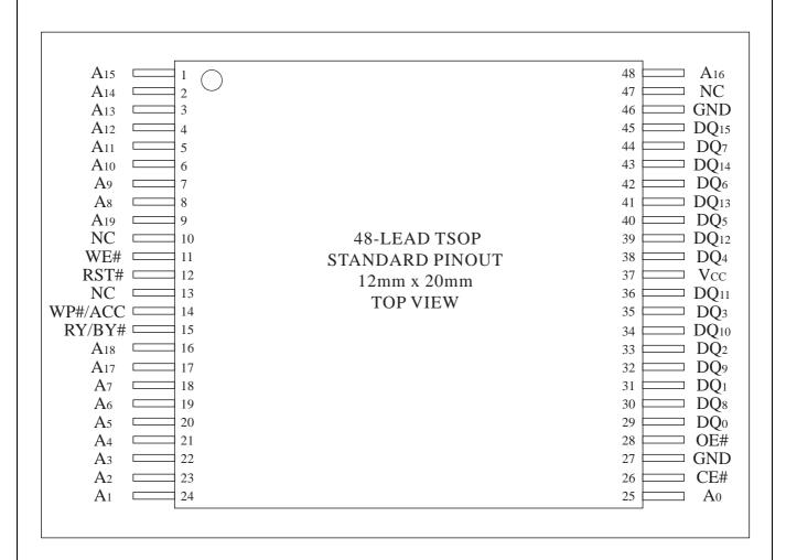
Figure 1. 48-Lead TSOP (Normal Bend) Pinout
