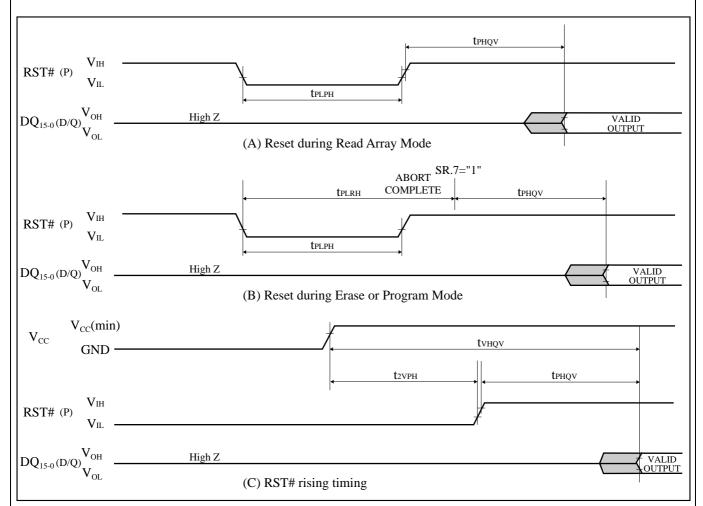
Figure 8. AC Waveform for Reset Operations
