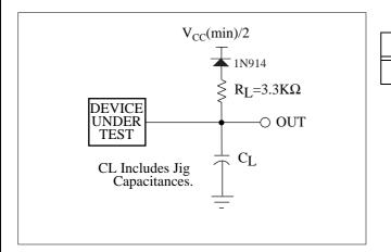
Figure 5. Transient Equivalent Testing Load Circuit
