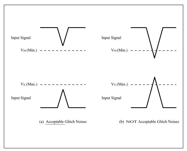
Figure A-2. Waveform for Glitch Noises
