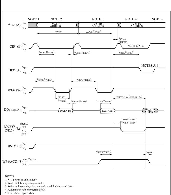
6. For read operation, OE# and CE# must be driven active, and WE# de-asserted.
