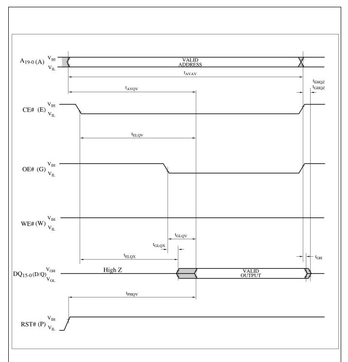
Figure 6. AC Waveform for Read Operations
