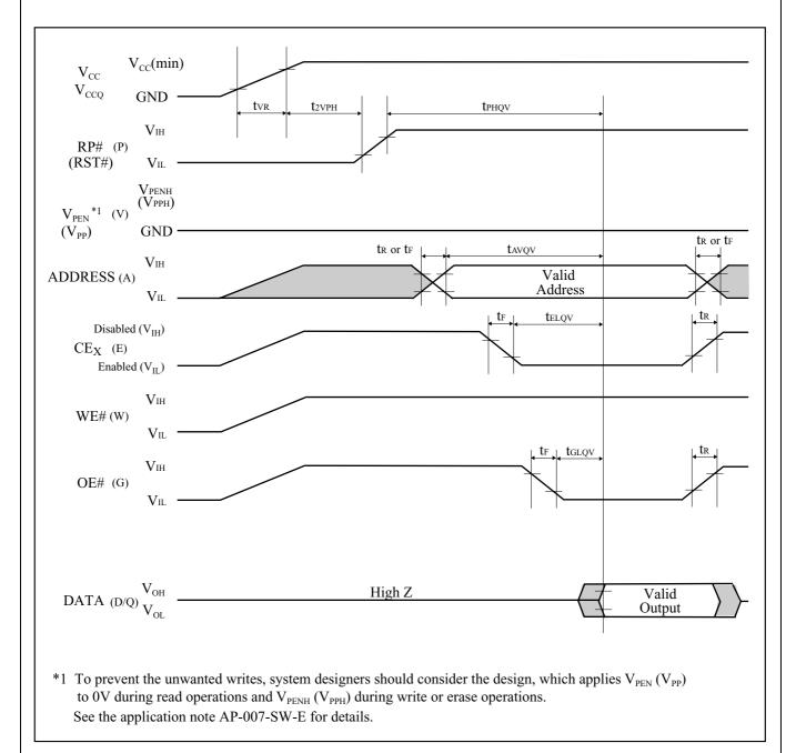
Figure A-1. AC Timing at Device Power-Up
