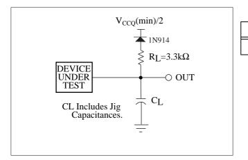
Figure 5. Transient Equivalent Testing Load Circuit
