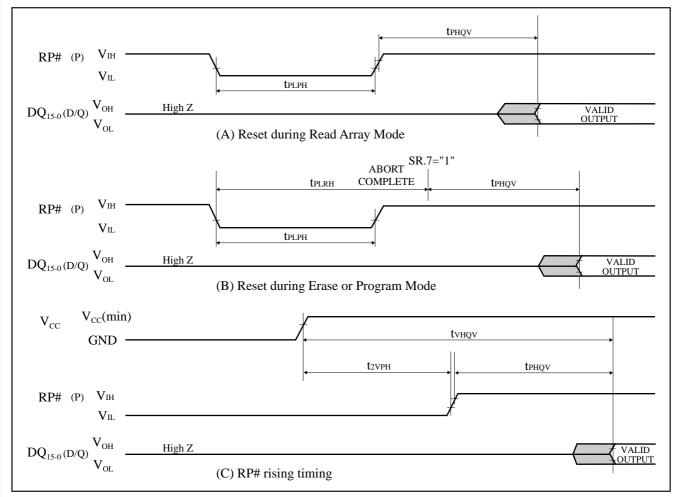
Figure 10. AC Waveform for Reset Operations
