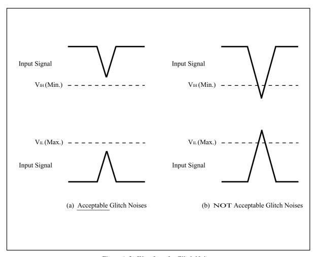
Figure A-2. Waveform for Glitch Noises
