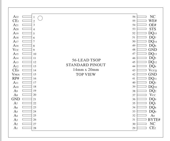
Figure 1. 56-Lead TSOP (Normal Bend) Pinout
