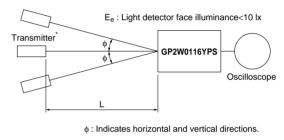
\* Transmitter shall use **GP2W0116YPS** (\(\lambda\)p=870nm TYP.) which is adjusted the radiation intensity at 3.6mW/sr
