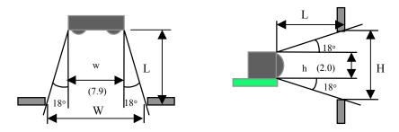
The optical window size should be the minimum size of W x H rectangular or elliptical in order not to reduce IrDA data transfer performance. The dimensions for W can be calculated by the formula of:
