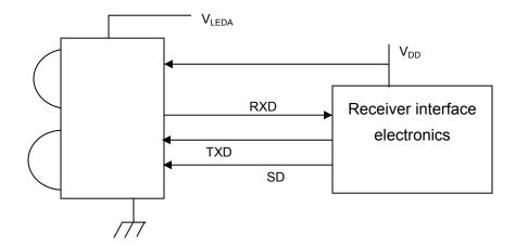
The  $V_{LEDA}$  voltage may be directly driven from the battery in the above design example. The  $V_{DD}$  associated with the Receiver interface electronics may be supported by a power regulator or other device providing an efficient regulated lower voltage source. This voltage may be as low as 2.0 Volts to 3.6 Volts, and the  $V_{LEDA}$  potential may range from 2.0 Volts to 6.0 Volts.
