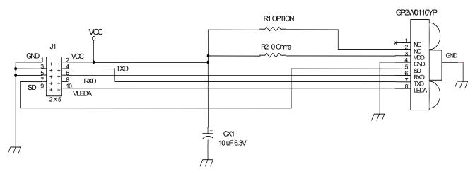
The value of capacitor CX1 is listed as 10  $\mu$ F. This value should be modified to meet your system electrical noise requirements. The decision should be based on the amount of system noise at the point where the IrDA transceiver will be powered. Both time-domain and frequency-domain noise issues should be considered. One common source of noise is switching power supplies, which need attention both on the power line and ground return paths.
