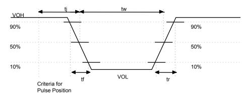
GP2W0110YP Infrared Transceiver Module Output Waveform
