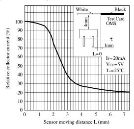
Fig.12 Relative Collector Current vs.
