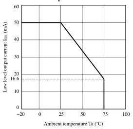
Fig.3 Low Level Output Voltage vs. Ambient Temperature
