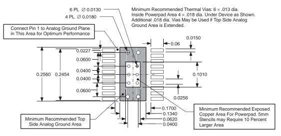
Figure 10. Recommended Land Pattern for 20-Pin PWP PowerPAD
