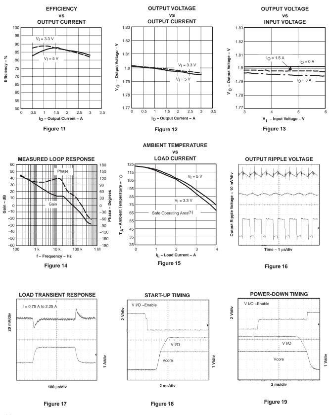
(1) Safe operating area is applicable to the test board conditions in the Dissipation Ratings
