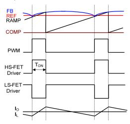
Figure 3: Heavy-Load Operation (PWM)
