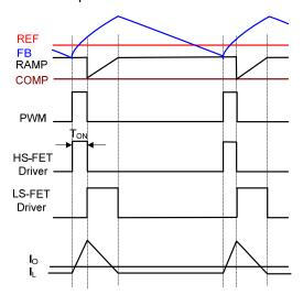
Figure 4: Pulse Skip at Light Load
