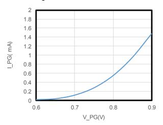
Figure 5: PGOOD Clamped Voltage vs. Pull-Up
