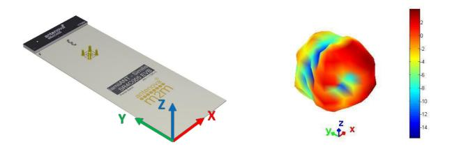
**3D pattern at 2580 MHz**Drag to rotate pattern and PCB by using Adobe Reader
