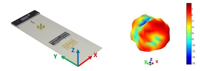
**3D pattern at 2340 MHz**Drag to rotate pattern and PCB by using Adobe Reader
