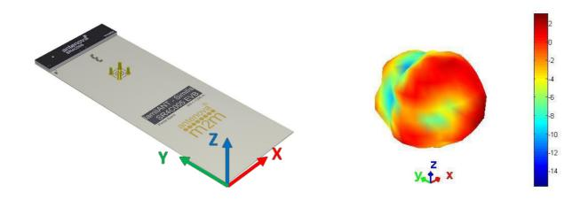
**3D pattern at 2110 MHz**Drag to rotate pattern and PCB by using Adobe Reader
