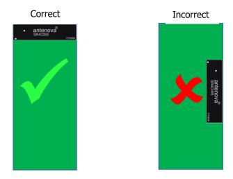
The antenna requires clearance ideally in 5 spatial directions as shown below. Where this cannot be achieved you should keep as many clear as possible to a minimum of 3. Please note performance will degrade with less clearances.
