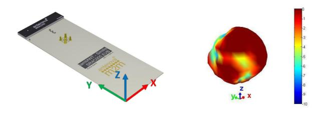
**3D pattern at 1810 MHz**Drag to rotate pattern and PCB by using Adobe Reader
