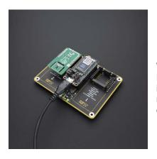
When USB mini connector is connected to the Feather base-board the PWR diode will glows Green, at this setup the Feather base board itself will be powered and will provide power to the shield including two mikroBUS sockets. The maximum current that Feather main board can provide over USB cannot exceed 500mA.
