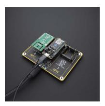
When USB type C connector is connected to the shield and USB mini connector is connected to the Feather base-board the PWR diode will glows Cyan, at this setup the mikroBUS sockets are powered from the Type C connector and Feather base-board is unloaded from delivering power to them. Feather base board is powered from his own source (USB mini) over which you can also upload program to your board.
