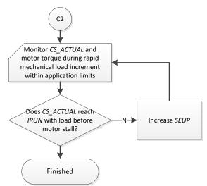
Figure 22.3 Enabling CoolStep (only in combination with SpreadCycle)
