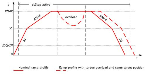
Figure 18.2 Velocity profile with impact by overload situation (example)
