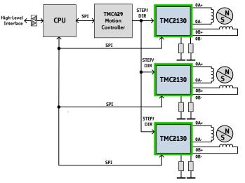
In this application, the CPU initializes the TMC2130 motor driver via SPI interface and controls motor movement by sending step and direction signals. A real time software realizes motion control.
