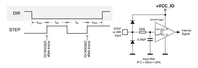
Figure 16.1 STEP and DIR timing, Input pin filter
