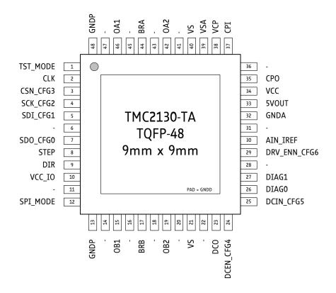
Figure 2.2 TMC2130-TA package and pinning TQFP-EP 48-EP (7x7mm<sup>2</sup> body, 9x9mm<sup>2</sup> with leads)
