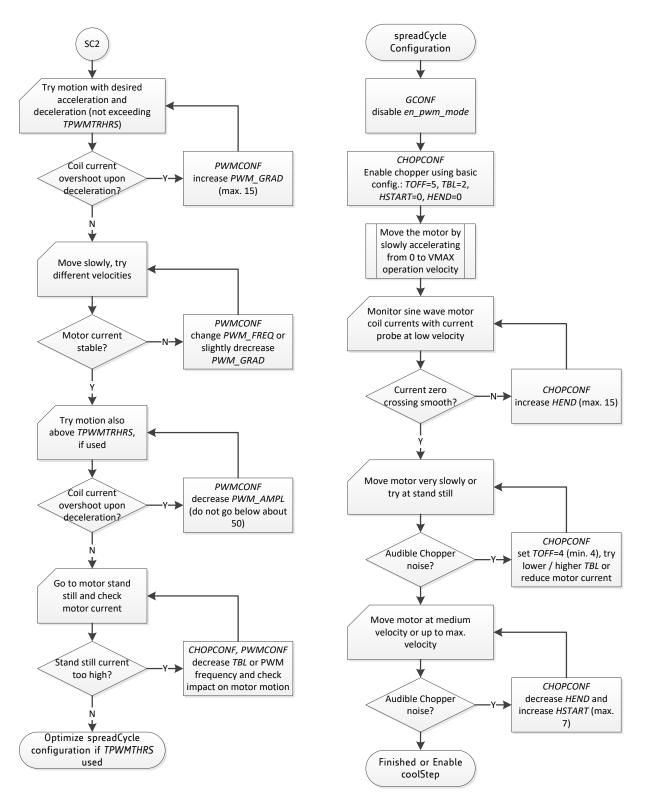
Figure 22.2 Tuning StealthChop and SpreadCycle
