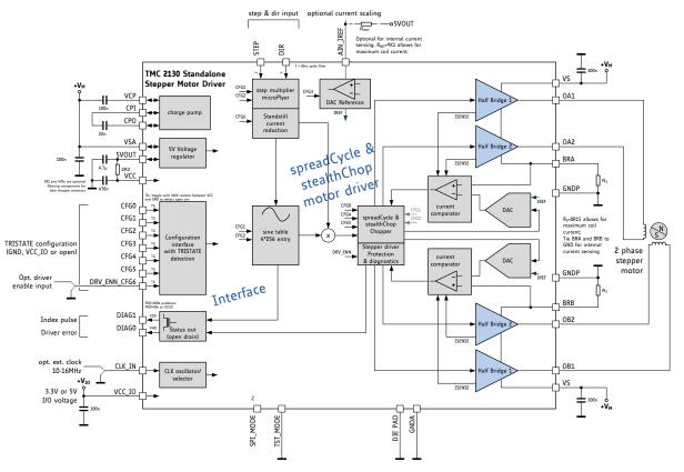
Figure 1.2 TMC2130 standalone driver application diagram
