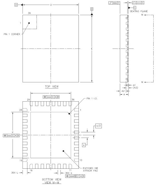
Figure 30.1 Dimensional drawings QFN 5x6
