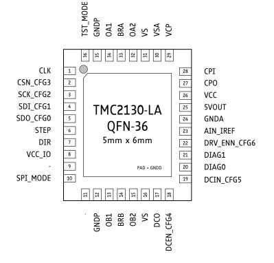
Figure 2.1 TMC2130-LA package and pinning QFN36 (5x6mm<sup>2</sup> body)
