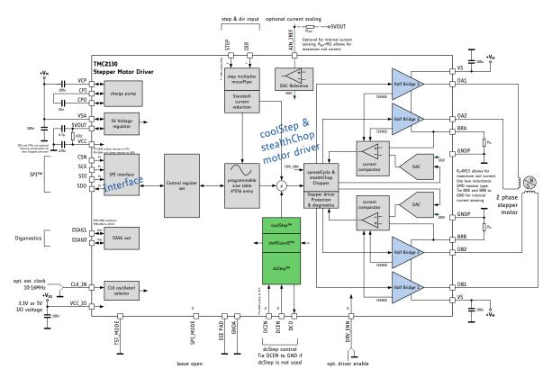
Figure 1.1 TMC2130 STEP/DIR application diagram
