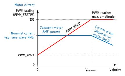
Figure 6.5 Velocity based PWM scaling (pwm\_autoscale=0)
