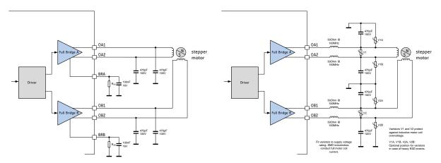
Figure 3.9 Simple ESD enhancement and more elaborate motor output protection
