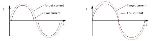
Coil current does not have optimum shape
