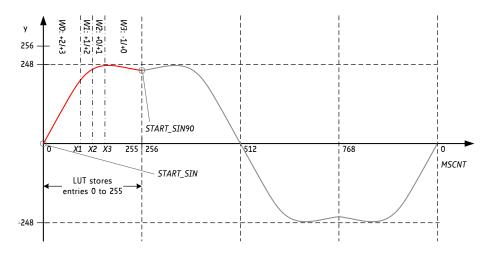
Figure 19.1 LUT programming example
