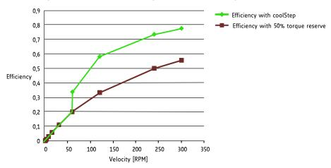
Figure 1.3 Energy efficiency with CoolStep (example)
