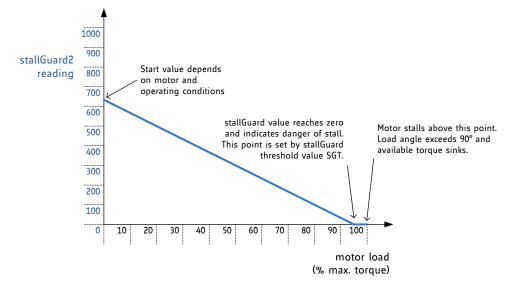
Figure 14.1 Function principle of StallGuard2
