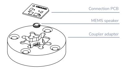
Figure 2: Coupler adapter assembly
