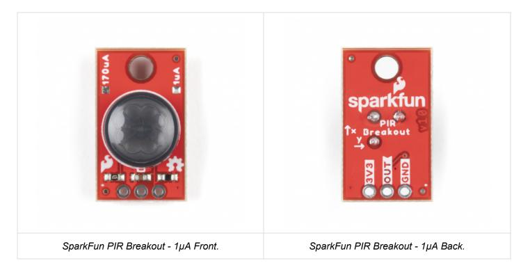
On each breakout we've broken the sensor's three pins (3V3/VDD, Ground and OUT) to a standard 0.1"-spaced PTH header for users to solder to. Take note that the sensors share the same PCB design and the version (**1µA** or **170µA**) is marked by the solder pads "North" of the PIR.
