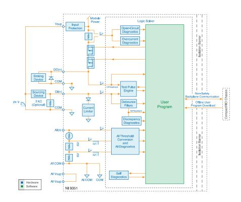
The analog input signals are scanned, amplified, conditioned, and then sampled by two independent ADCs. The module provides overvoltage protection for each channel. Only one channel can be in an overvoltage condition at a time.
