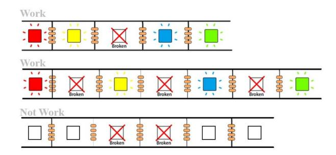
As long as not two or more adjacent LEDs are broken, the remaining LEDs will be able to work normally
