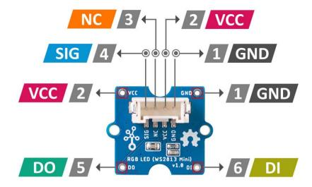
1 : Connected to the system GND
