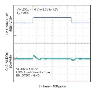
Figure 6. TPS650001/3/6 LDOx Line Transient Response
