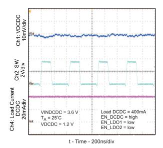
Figure 8. TPS650001/3/6 Output Voltage Ripple (MODE = high)
