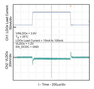
Figure 4. TPS650001/3/6 LDOx Transient Response
