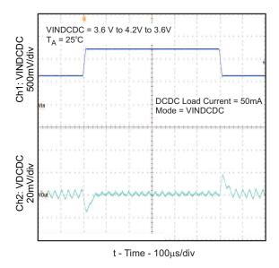
Figure 5. TPS650001/3/6 DCDC Converter Line Transient Response
