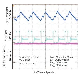
Figure 7. TPS650001/3/6 Output Voltage Ripple (MODE = low)
