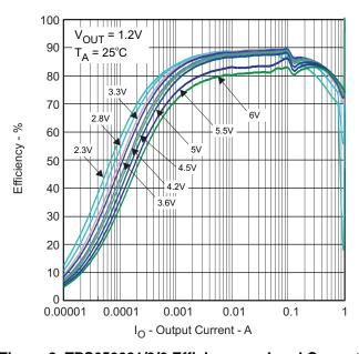
Figure 2. TPS650001/3/6 Efficiency vs Load Current
