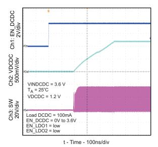
Figure 9. TPS650001/3/6 DCDC Converter Startup Timing
