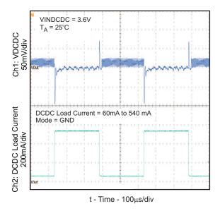
Figure 3. TPS650001/3/6 DCDC Converter Load Transient Response
