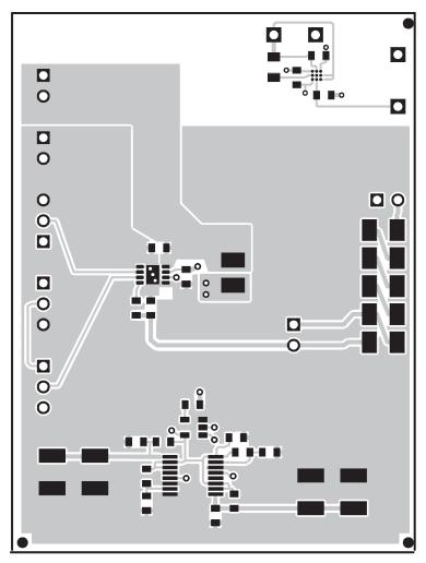
Figure 2. Top Layer Routing
