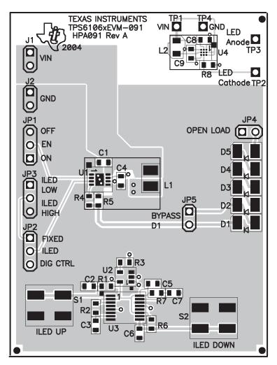
Figure 1. Top Assembly Layer
