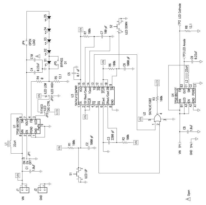
Figure 4. TPS6106xEVM Schematic
