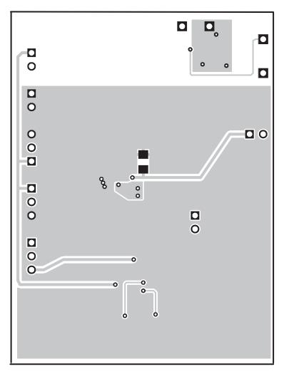
Figure 3. Bottom Layer Routing
